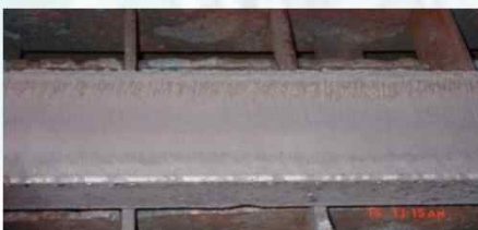
Cutting quality of Gwangyang Iron Company (thickness: 230 mm )
