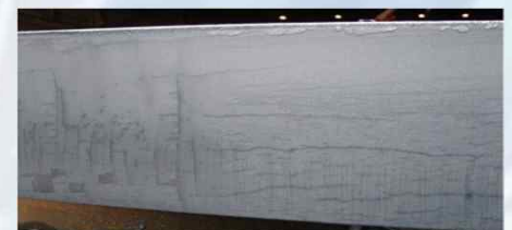
Cutting quality of Corus Corporation in Netherlands (thickness: 230 mm / speed: 220mm/min )
