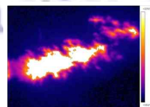
Compound combustion of paraffin oil and Hydrox (6 m 3 /hr)
