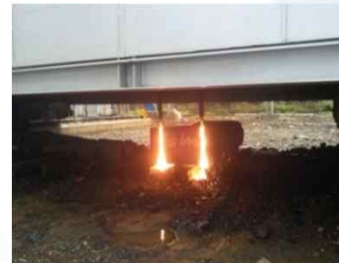
Special Steel Cutting by 2 torches in POSCO 600mm E-160M
