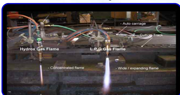
Structure of cutting flame
