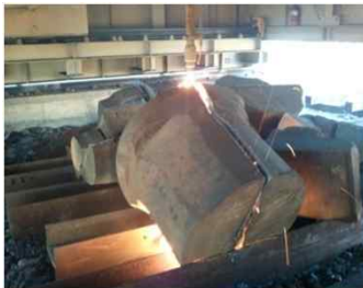
Special Steel Cutting in POSCO 500~1,000mm E-160M
