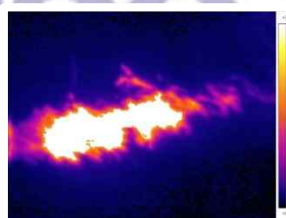
Compound combustion of paraffin oil and Hydrox (3 m 3 /hr)
