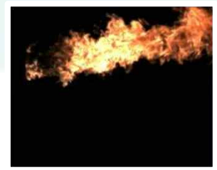
Compound combustion of paraffin oil and Hydrox (6 m 3 /hr)
