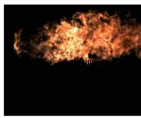
Compound combustion of paraffin oil and Hydrox (3 m 3 /hr)
